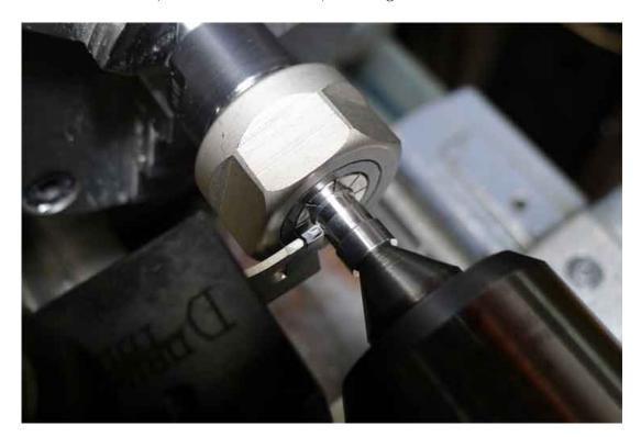
(3) Do not deburr or polish the newly cut sharp edges of the grooves.
