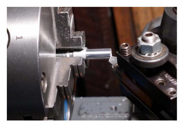
4. With the dial indicator, move the cutter a small distance toward the lathe chuck and cut the body of the ferrule to length.
