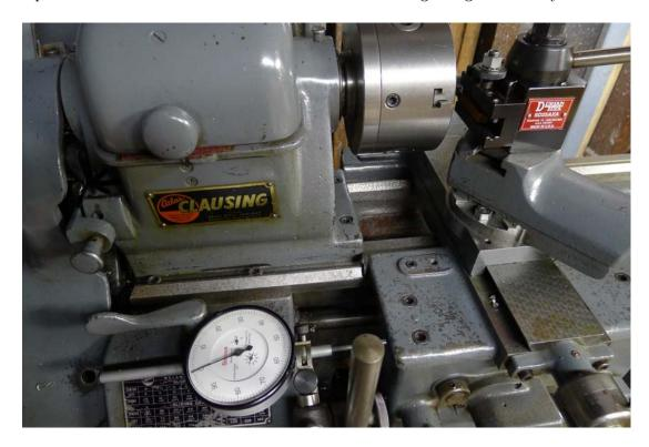
3. Align the cutter with a slight  $90^{\circ}$  back angle to ensure a square shoulder cut. Cut the body to the desired diameter.
