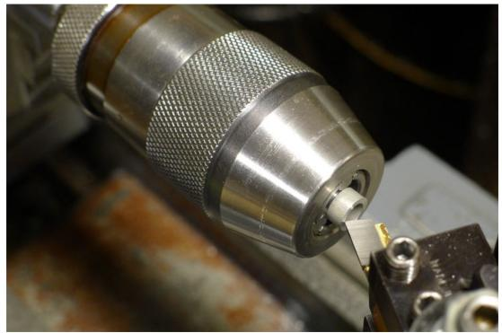
9. On a drill press, deburr the head hole by hand-feeding the ferrule into a slowly rotating countersink.
