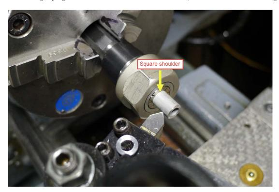
8. Insert a Morse taper extension into the lathe spindle and mount a keyless chuck. With the dial indicator, turn a very fine 0.002 in. finish cut on the head of the ferrule.
