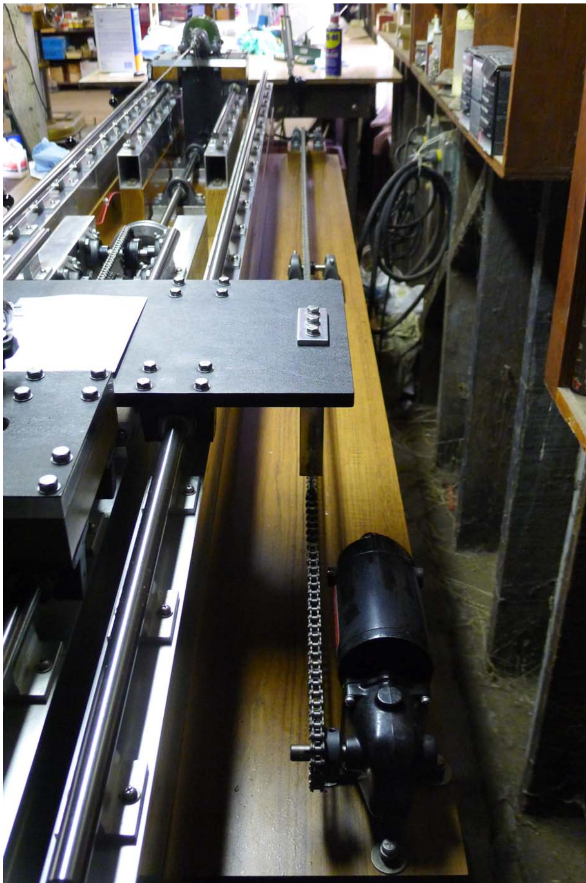
Variable speed DC gearmotor and chain that drive the spool carriage.
