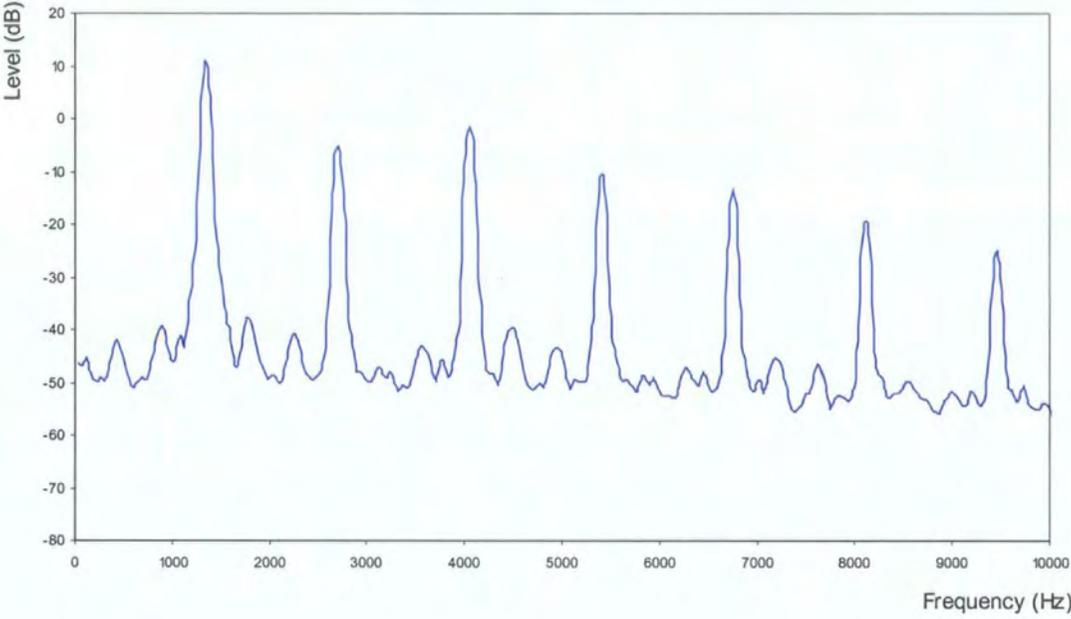
Figure 6-18 Spectrum of E<sub>6</sub> on the Boehm Flute
