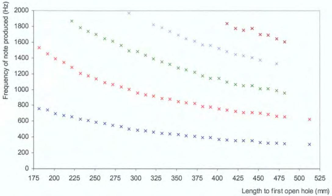
Figure 8-6 Frequencies produced at different lengths on the 14mm sieve flute
