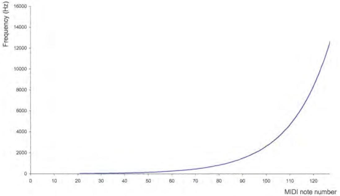
**Figure 3-1 Frequencies of 12 Equal-Tempered Tuning**
