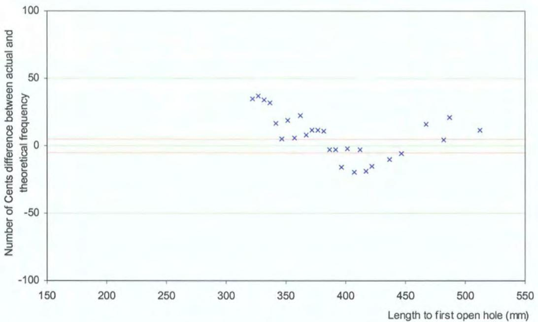
**Figure 8-22 Comparison of the number of cents away from the theoretical frequencies for the 3<sup>rd</sup> Overblown frequencies with modified end effect**
