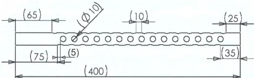
Figure 8-4 Dimensions of 10mm sieve flute
