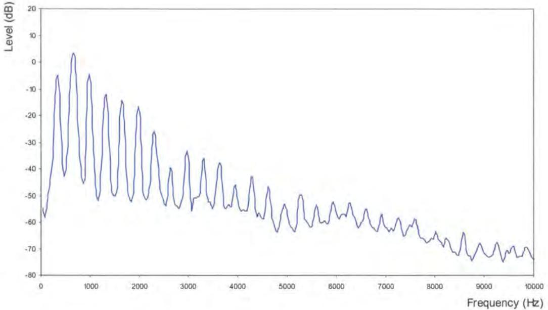
Figure 7-3 Spectrum of E<sub>4</sub> on the Boehm Flute
