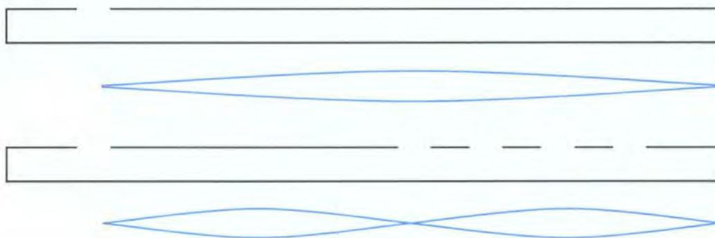
**Figure 2-4 Fundamental waves on a flute**
