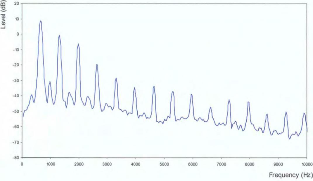
Figure 6-17 Spectrum of E<sub>5</sub> on the Boehm Flute
