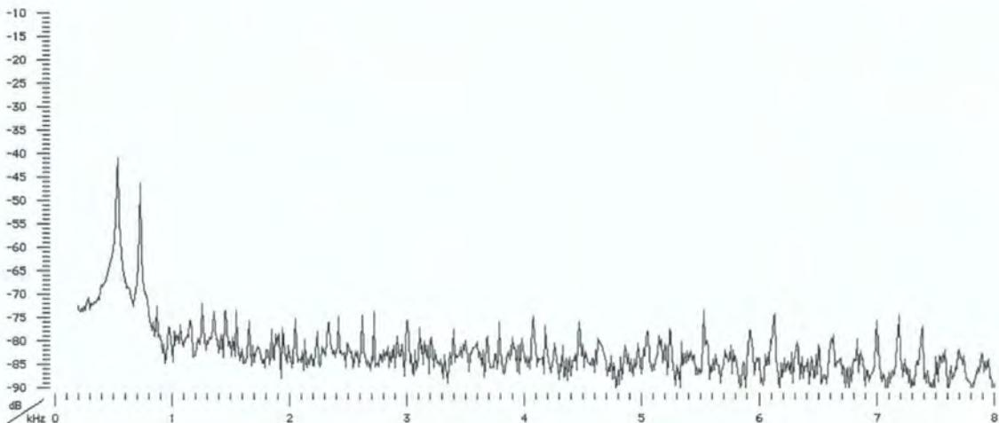
Figure 2-8 The spectrum of a Multiphonic ( $C_5$  and  $F\#_5$ ) on the flute<sup>10</sup>
