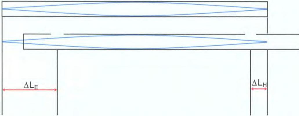
**Figure 2-6 Flute's acoustical length a tone hole open.**
