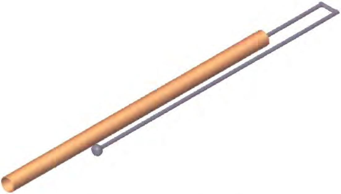
Figure 7-7 Modified design of plunger flute
