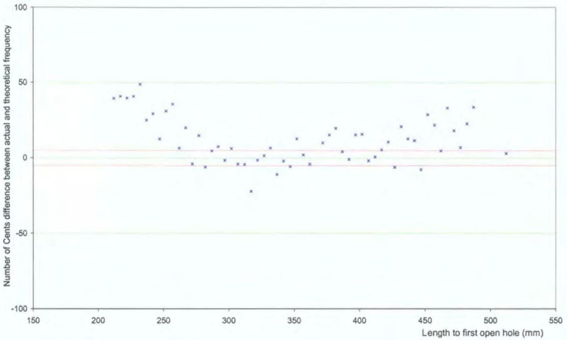
**Figure 8-21 Comparison of the number of cents away from the theoretical frequencies for the 2<sup>nd</sup> Overblown frequencies with modified end effect**
