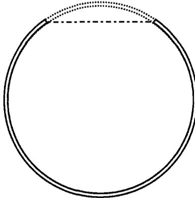
**Figure 8-5 cylindrical bore without chimneys becoming non-cylindrical**
