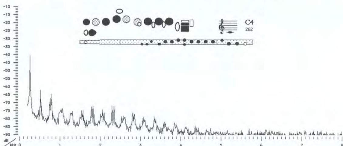
Figure 2-11 The Sound Spectrum for C<sub>4</sub> being played pianissimo on a flute.<sup>13</sup>
