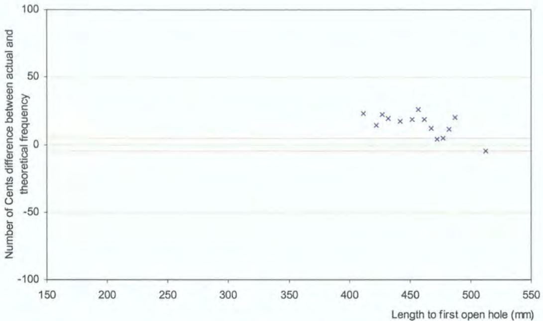
**Figure 8-23 Comparison of the number of cents away from the theoretical frequencies for the 4<sup>th</sup> Overblown frequencies with modified end effect**
