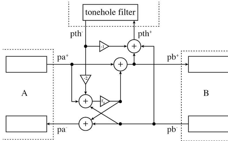
Figure 5: Air pressure scattering at the tonehole location [17] [4].
