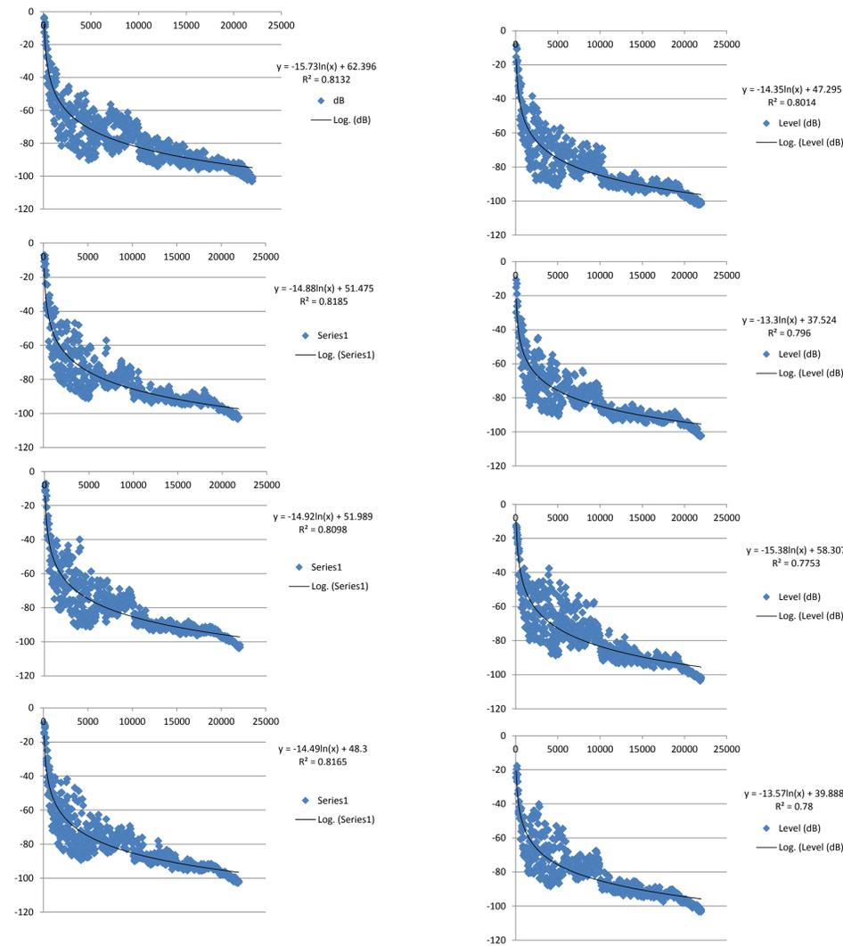
These are graphs of HCS ratings. Hz are displayed on the x-axis, and dB are displayed on the y-axis.
